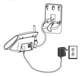
1 Insert the four tabs on the wall mount into the four slots on the back of the base and push down.
